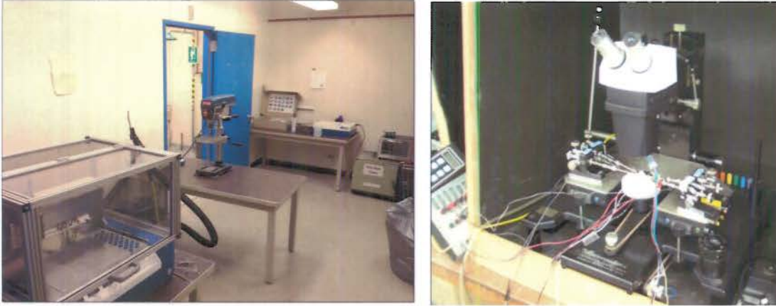
The UH Fabrication Lab (left) houses numerous Making tools. In one project for the Navy (right), a temperature controlled platform was 3D printed by graduate student, Trent Robertson, to fit a micromanipulator stage that feeds into a semiconductor parameter analyzer for testing chips.
